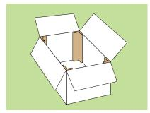
The strength of a single package can be improved by reinforcing boxes internally with edgeboards.
