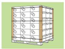
Edgeboards stabilise the pallets and provide protection during transport and warehousing.
