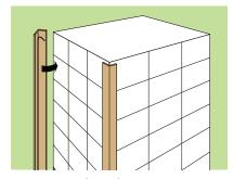
The use of self-adhesive edgeboard improves handling before final strapping is applied.
