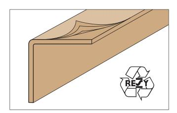
Raw Material. The standard edgeboard is manufactured by laminating several layers of strong paperboard.
