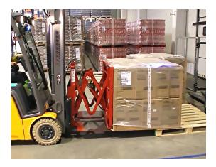
**Case study:** Palletless handling for export Customer had a high freight cost in overseas shipments. They wanted to try palletless handling instead of using wooden pallets to be able load more goods per container.
