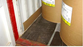
Uneven walls and floors in containers and trains may cause transport damage to the loaded goods. This can be avoided by using Flatboards as side and floor protection.
